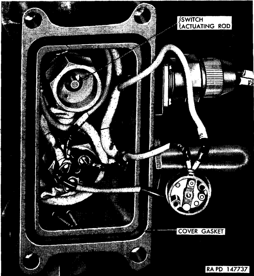
Figure 203. Engine oil cooler fan controller—low temperature switch removed.
